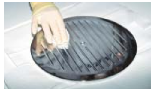
5) You want every impurity out of the pores of the metal because Zoopseal is going to fill those pores and maintain the exact appearance that you start out with on the part.
