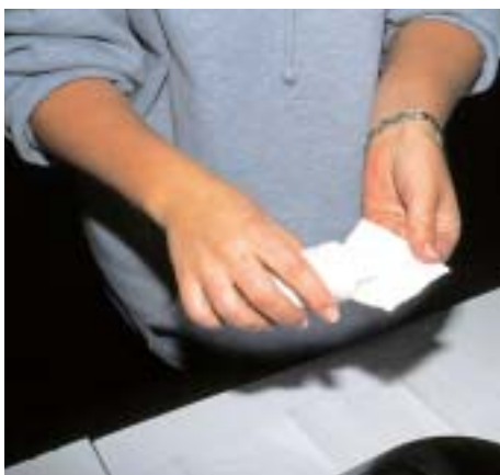
7) Dip the cloth in the seal, and you're ready to start coating the part.
